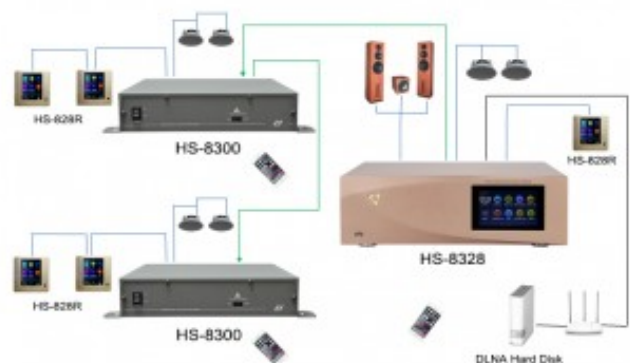
HS-8328 System Connection Diagram
