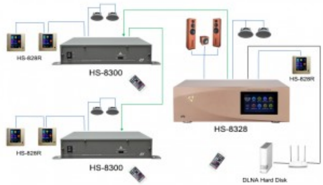
HS-8328 System Connection Diagram
